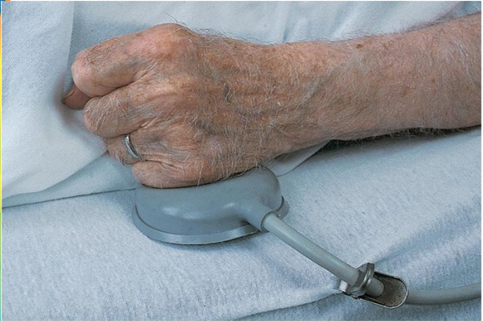
Fig. 14-14. Signal light for a person with limited hand mobility.
